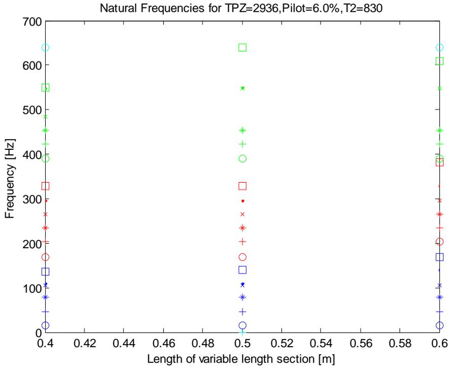
**Figure 2:** Thermo-acoustic network natural frequency prediction.
