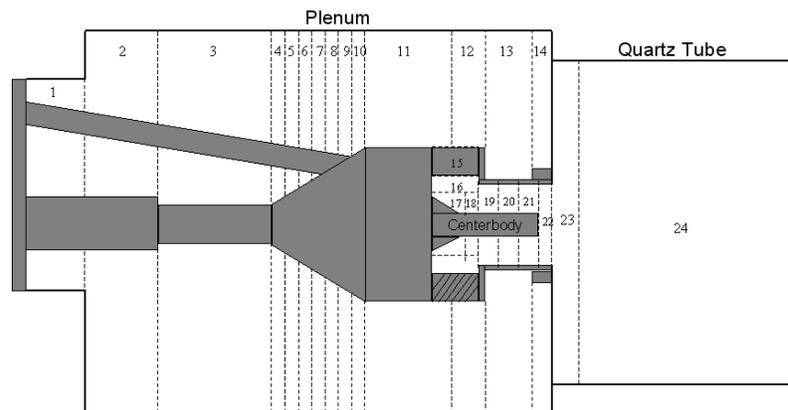
**Figure 1:** Model illustration with each duct separated by dashed lines.
