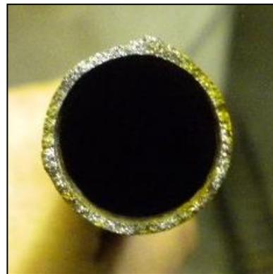
After performing a calculation at the location of the fracture (a raised shoulder) the igniter was seen to have a minimum yield strength of 25 ft-lbs of torque. This assumes Maximum Shear Stress Model, worst case material properties, and maximum stress concentration factor for the geometry. While this calculation shows a yield strength of 5 ft-lbs less than the tested yield
