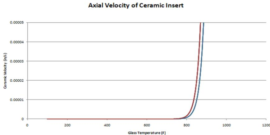
This plot shows that for two different loading schemes, represented by red and blue lines, the glass becomes soft enough at a temperature of 800 F to experience an appreciable amount of ceramic drift. This is a reasonable temperature for the igniter tip to see.
