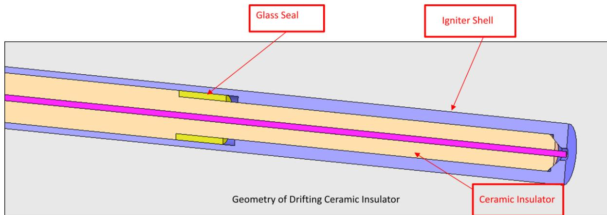
One concern with this design is that the ceramic insulator may recess, or drift, away from the surface of the shell. This 'drift' of the ceramic insulator away from its seat will result in a loss of the preload that the ceramic was designed to be under. This would not affect the functionality of the part, but it does leave the part more open to damage since an unsupported ceramic is more likely to crack when jostled.
