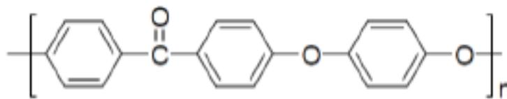
Figure 5. Chemical structure of PEEK
