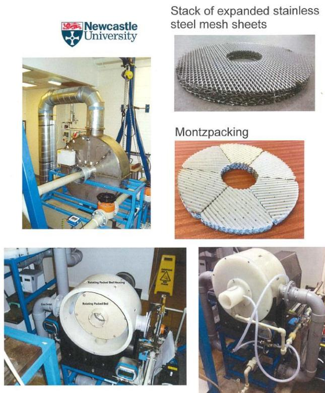
Figure 4. Produced rotating packed bed reactors and interior packing (Newcastle University)
