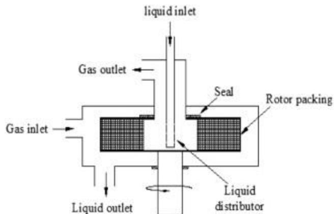
Figure 1. The basic design of the rotating packed be reactor.<sup>5</sup>
