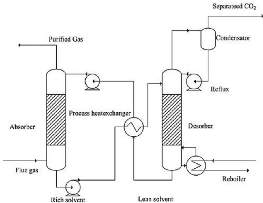
Figure 3. A simplified PFD for a traditional carbon capture system. In the ROTA-CAP system the traditional absorber and desorber will be replaced with RPBs.<sup>7</sup>
