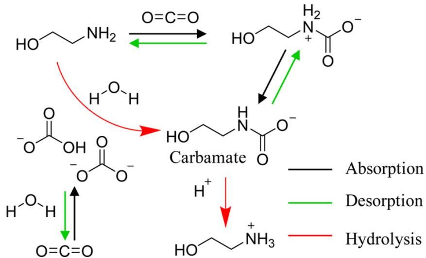
Figure 2: Reaction of typical amine MEA with carbon dioxide for absorption or desorption.<sup>6</sup>
