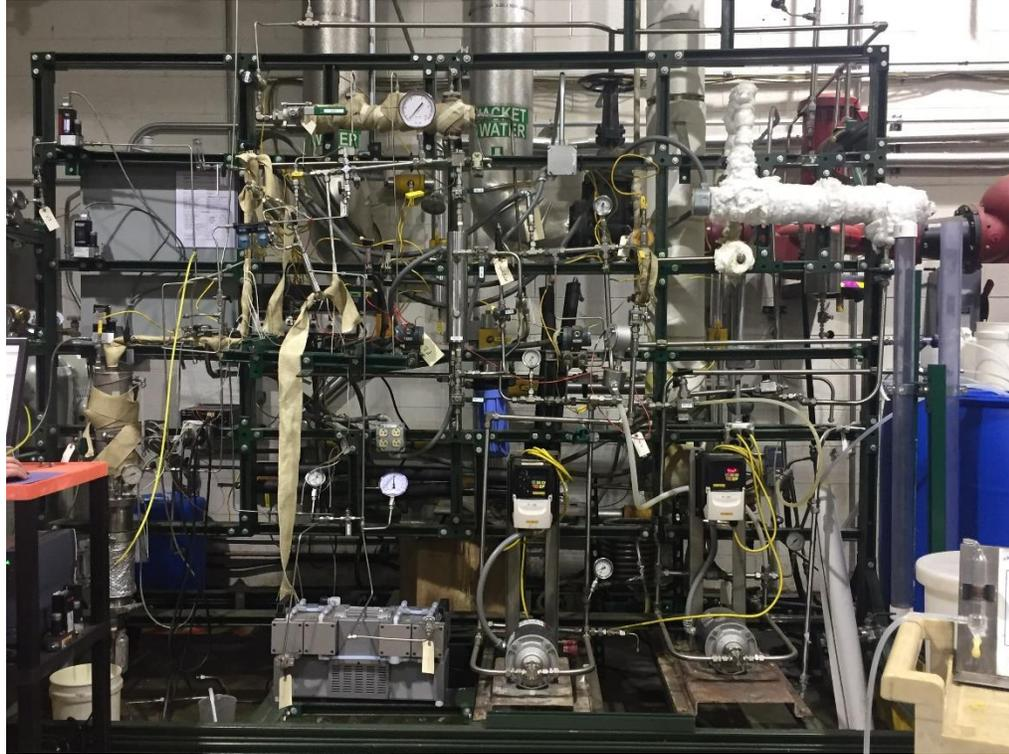
Figure 6. GO-PEEK membrane apparatus.
