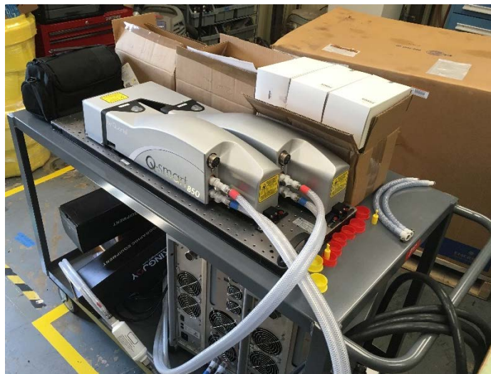
Figure 4. Laser Mounted to Cart, Cooling Units Below
