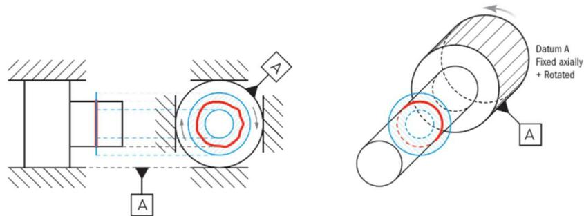
Fig 5: Runout feature measurement<sup>1</sup>
