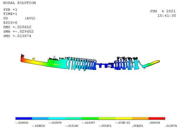
Fig 6: Ansys plot of a unit gravity sag model
