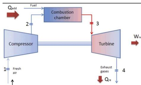
Fig 7: Flow diagram of the turbine engine
