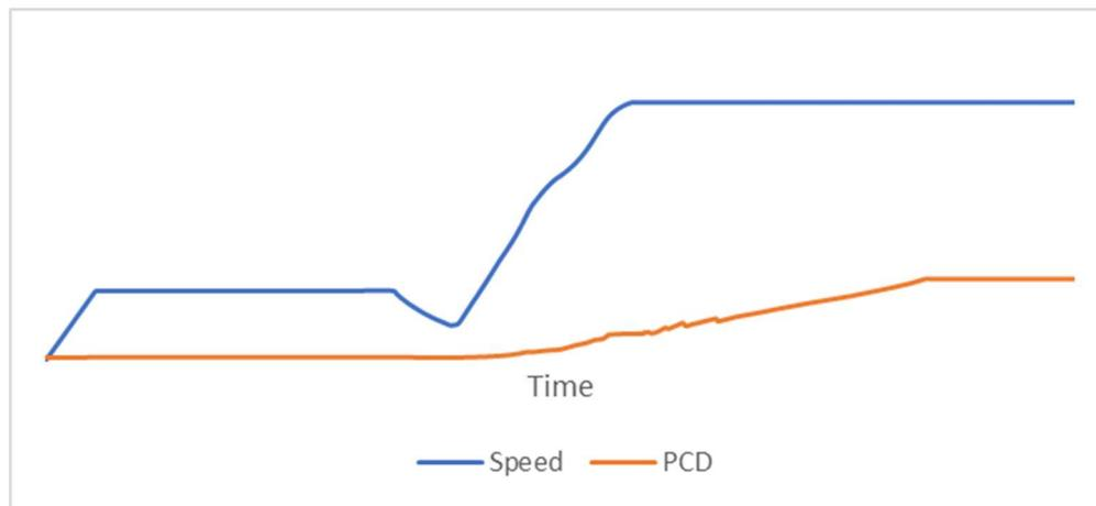
Fig 1. Typical compressor discharge pressure and speed versus time. (Graph not to scale due to confidentiality)
