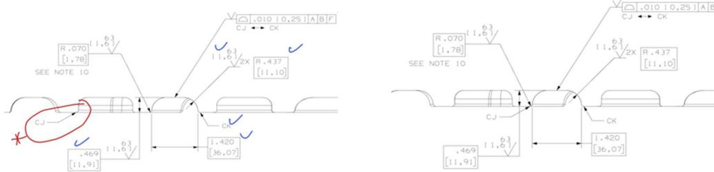
Fig 3: Dimensioning error over surface profile CJ-CK left image compared to the right
