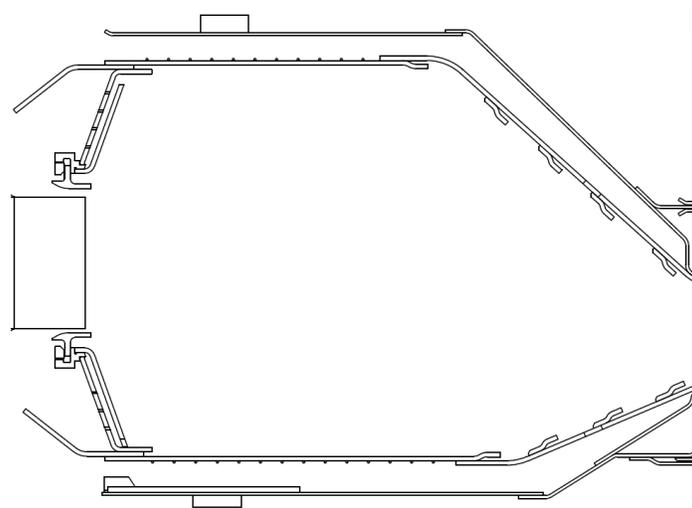
Figure 1: Combustor liner used in popular Solar Turbines engine
