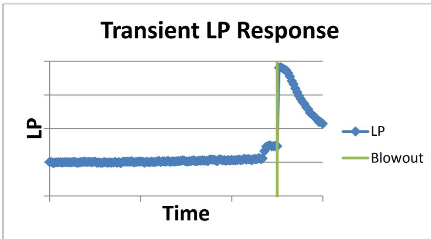
Figure 4 - Transient response of LP during a blowout with no pilot
