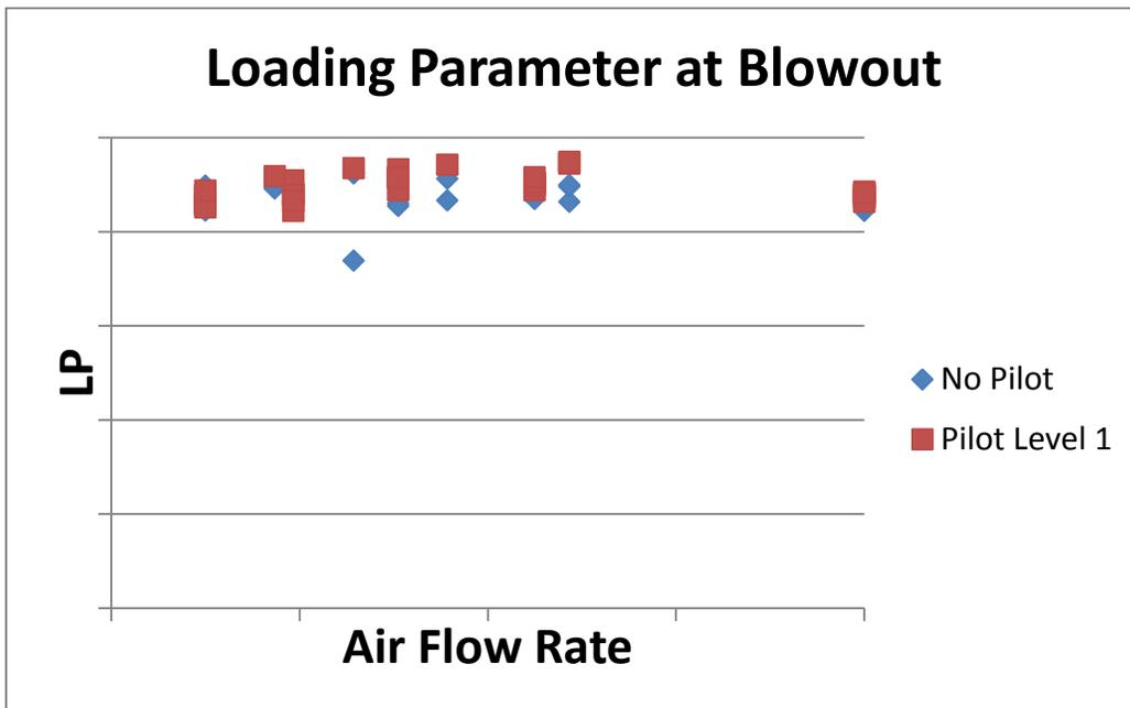
Figure 2 - Combustor Loading Parameter versus air flow at blowout conditions
