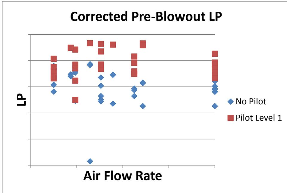
Figure 6 – Corrected combustor LP versus air flow at conditions immediately before blowout
