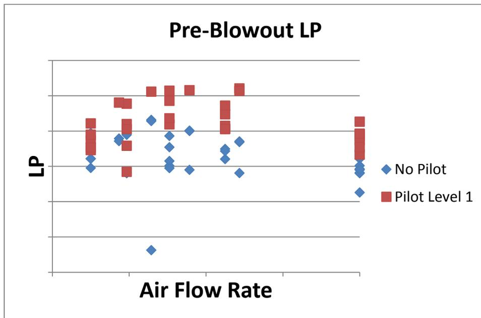
Figure 5 – Combustor LP versus air flow at conditions immediately before blowout
