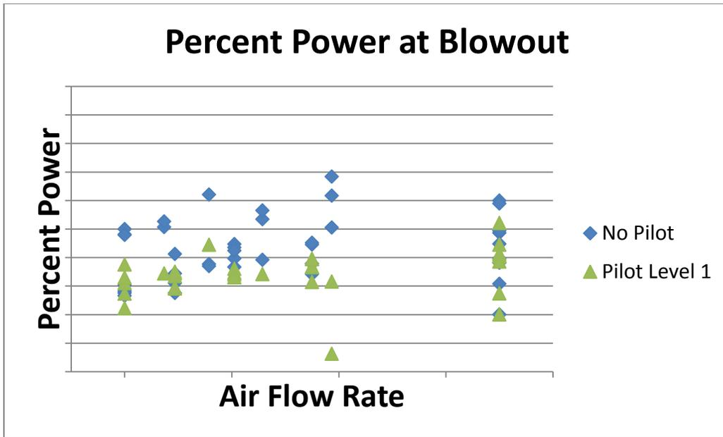
Figure 1 - Output percent power versus air flow at blowout conditions
