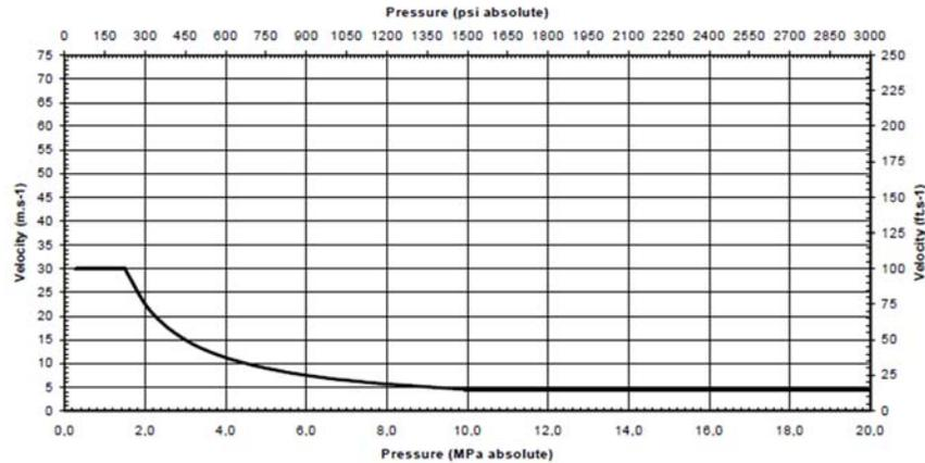
**Figure 9. Impingement velocity curve for carbon steel at 150° C and stainless steel at 200° C (IGC Doc 13/12/E)**
