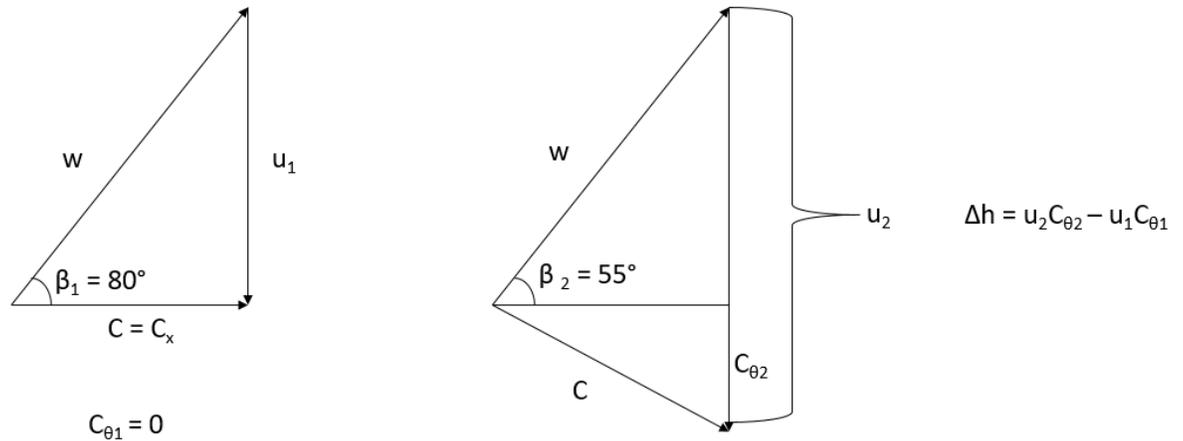
**Figure 4. Velocity triangles (not to scale)**
