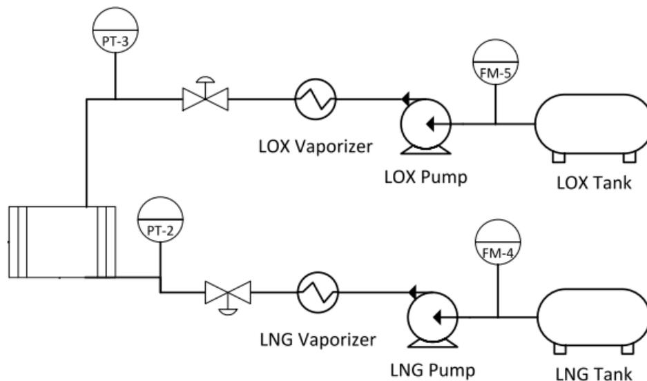
**Figure 8. Piping and instrumentation diagram of LOX and LNG delivery**
