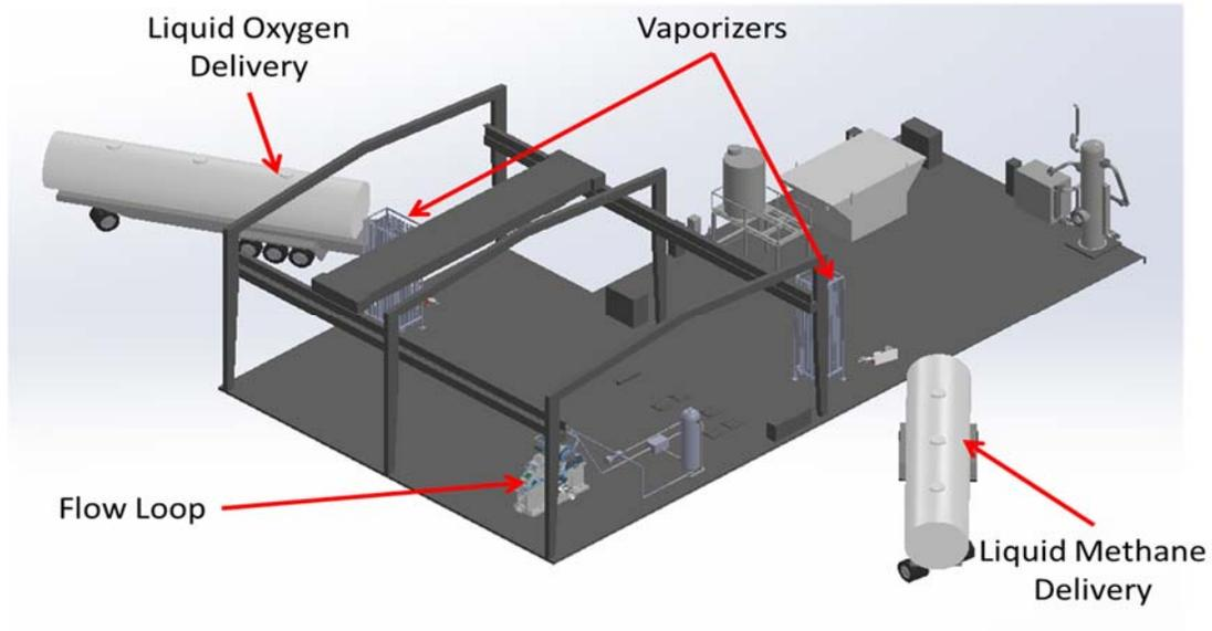
**Figure 7. Reduced flow test loop layout**
