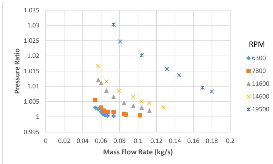
**Figure 6. Compressor map of test demo using experimental data**
