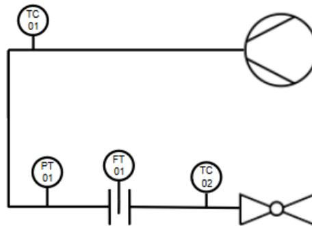
**Figure 2. Piping and instrumentation diagram of axial compressor test demo**
