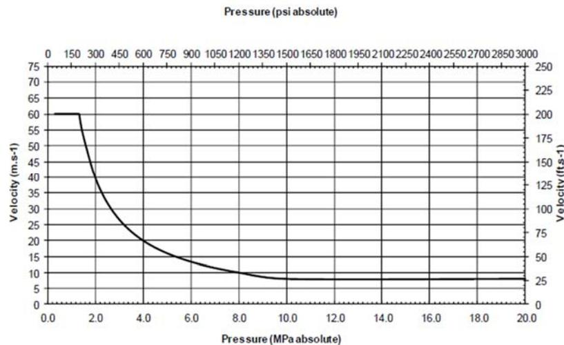
**Figure 10. Non-impingement velocity curve for carbon steel at 150° C and stainless steel at 200° C (IGC Doc 13/12/E)**
