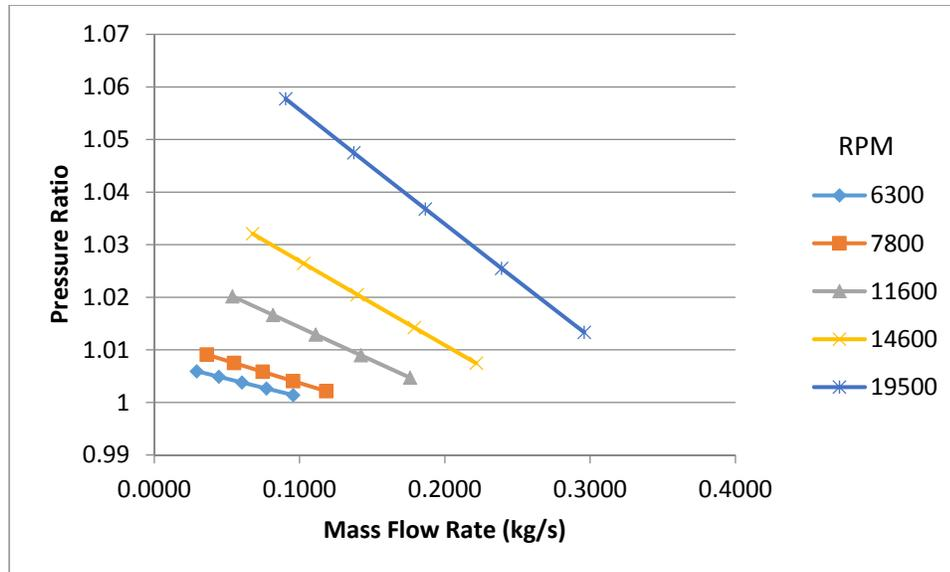
**Figure 5. Theoretical compressor map of test demo**
