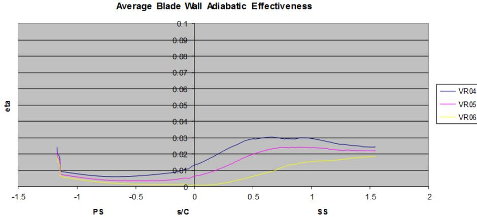
Figure 3.3: Adiabatic wall effectiveness for three velocity injection ratios.
