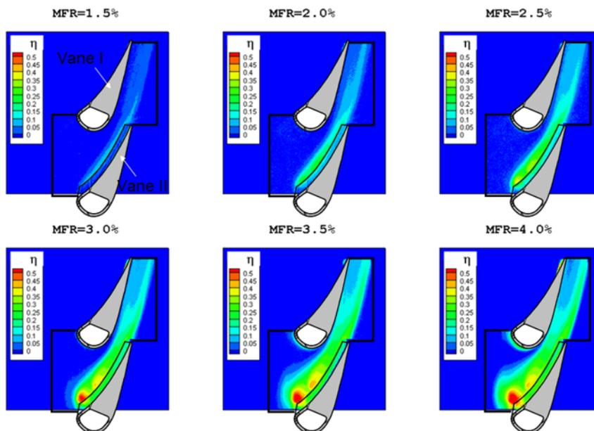
Figure 2.3: Endwall adiabatic wall effectiveness for vane I showerhead and suction side injection, and vane II showerhead and pressure side injection.
