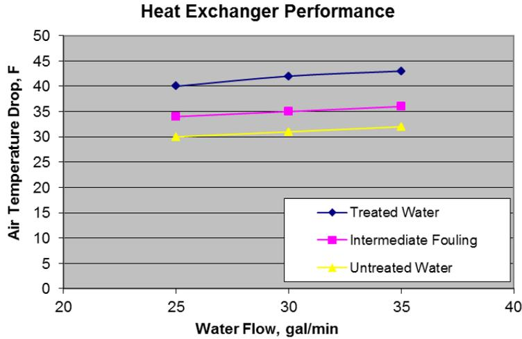
Figure 2.6: Heat exchanger temperature drop for various water flow rates and fouling factors.
