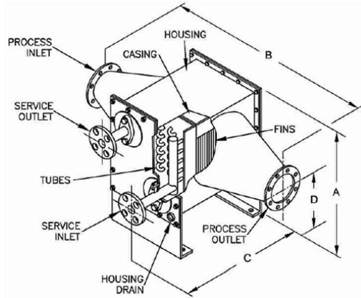
Figure 2.4: Xchanger Inc., C-275 Fin-Tube Core Heat Exchanger.
