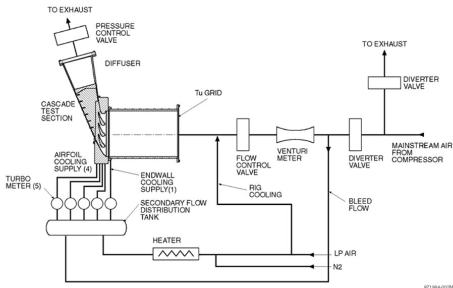
Figure 2.2: Schematic of scaled cascade rig.
