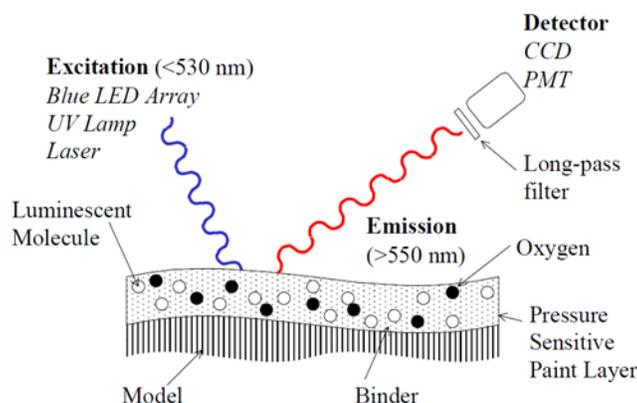
Figure 2.1: A pressure sensitive paint detection system.
