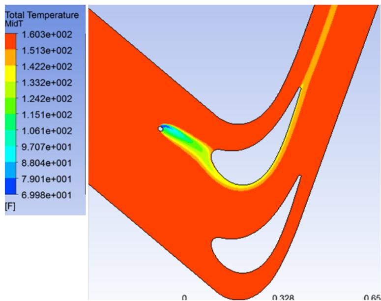
Figure 3.2: Temperature contour at blade mid-span for cooling hole three activated.
