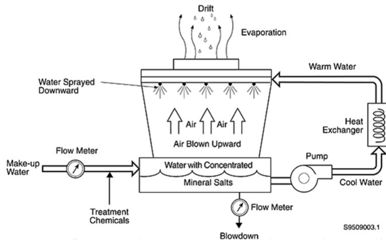
Figure 2.5: Schematic of the cooling tower water loop and operation.
