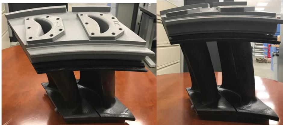
FIGURE 5. Full-scale model of the Stage 2 CMC nozzle.
