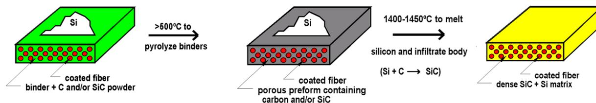
FIGURE 2. Process for strengthening and finishing the final CMC part.
