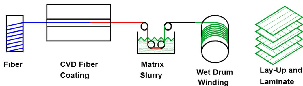
FIGURE 1. Process to create sheets of CMC material.
