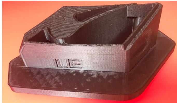
FIGURE 7. ABS part not treated in acetone.
