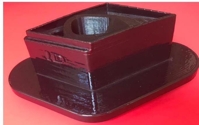
FIGURE 8. ABS part treated using acetone.
