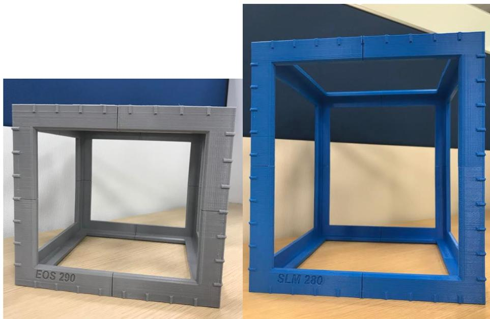
FIGURE 9. Boxes that represent the build volume of the EOS 290 and the SLM 280.
