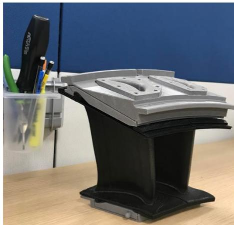
FIGURE 4. Half-scale model of the Stage 2 CMC Nozzle.
