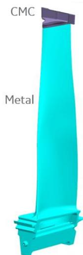
FIGURE 6. Last stage blade example, with CMC tip.
