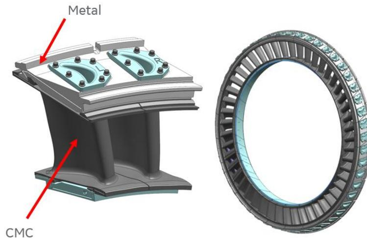
FIGURE 3. Stage 2 Nozzle model.
