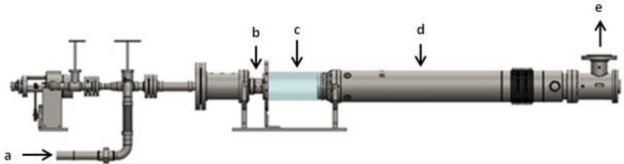
**Figure 2: PSU test rig schematic: a) Inlet air – Flow direction is from left to right; b) Solar Turbines Taurus 70 injector; c) Quartz combustor section -- Quartz window allows optical access to the flame; d) Stainless steel combustor section – The axial location of a plug inside this section can be varied**
