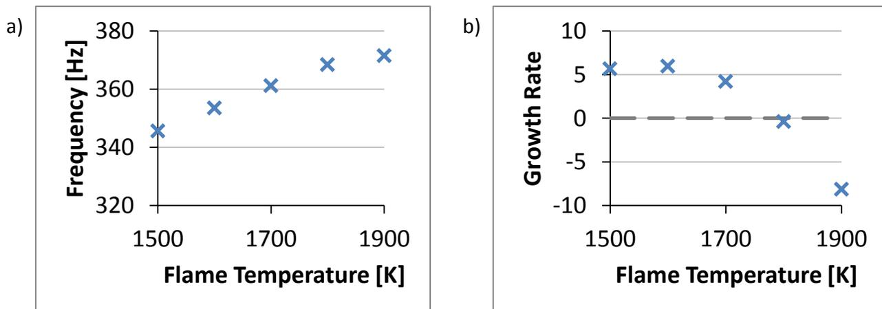
**Figure 6: a) Frequency and b) Growth Rate predictions for  $L_{\text{comb}} = 41\text{in}$
