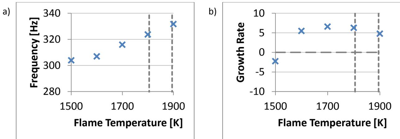
**Figure 8: a) Frequency and b) Growth Rate predictions for  $L_{comb} = 41in$
