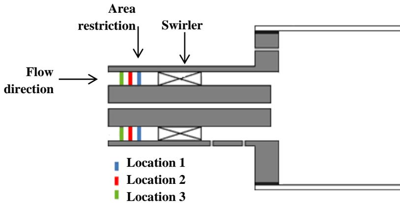
**Figure 3: Schematic of the Taurus 70 injector in the PSU rig. Colored lines indicate the location of the inlet area restriction**
