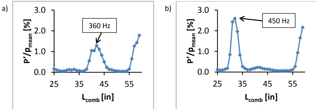
**Figure 5: PSU rig stability maps with instability frequency indicated**
