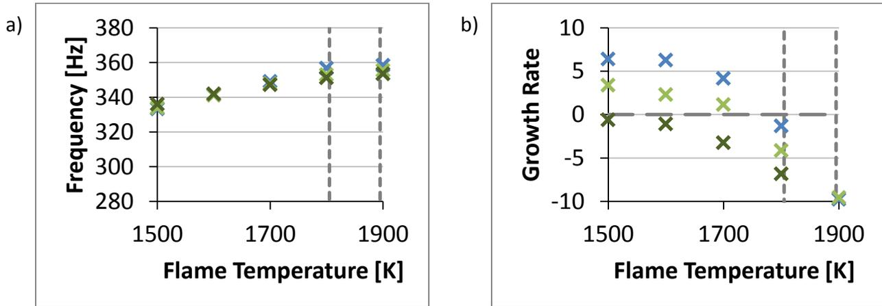
**Figure 12: Effect of velocity component phase on model results. The blue, light green, and dark green x's indicate phase values of  $0^\circ$ ,  $20^\circ$ , and  $40^\circ$  respectively**
