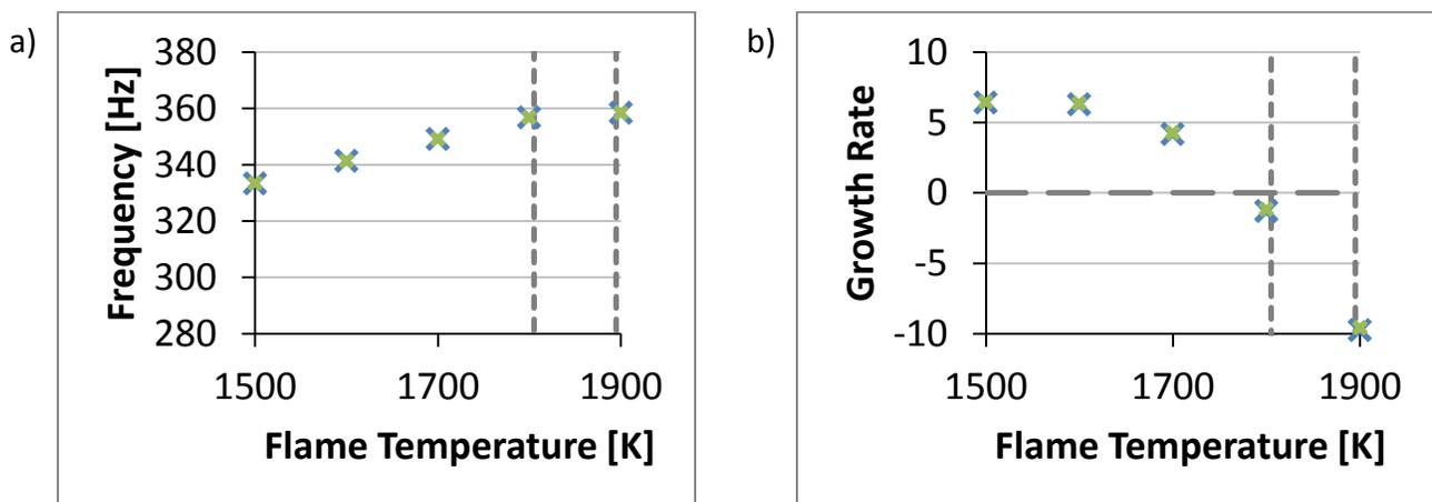
**Figure 11: Predicted frequencies and growth rates with the area restriction in the original location (blue) and 2in. upstream (green)**
