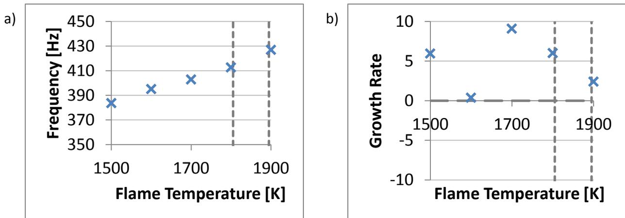
**Figure 9: a) Frequency and b) Growth Rate predictions for  $L_{comb} = 32in$
