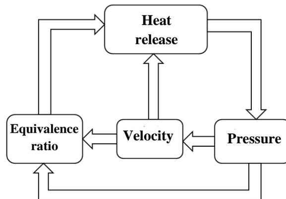
**Figure 1: Combustion oscillation feedback loop**
