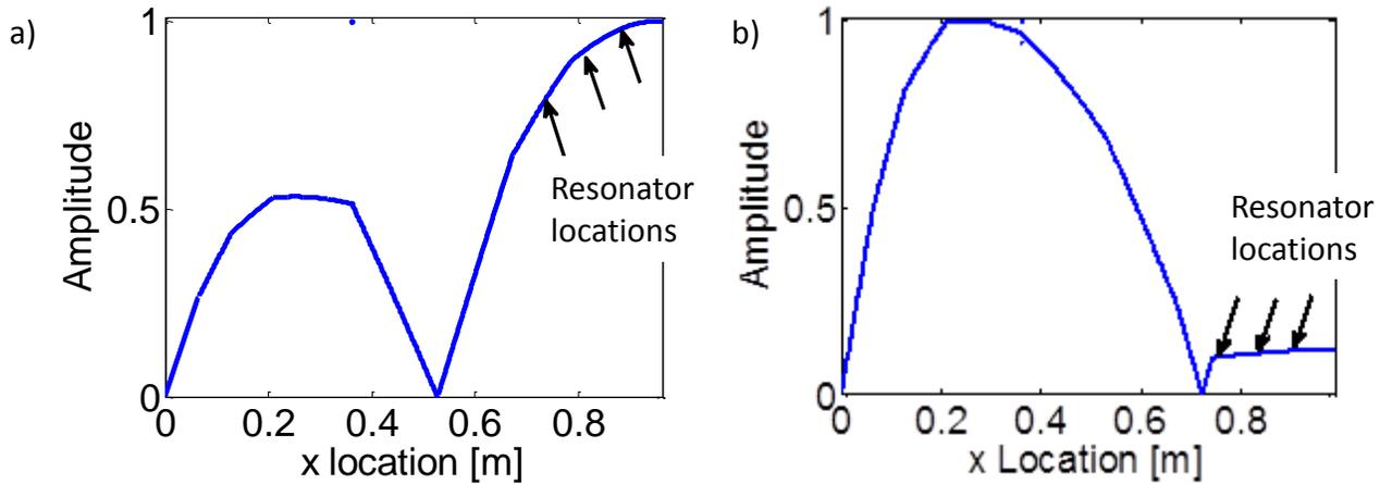
**Figure 13: 200 Hz natural frequency mode shapes for the Taurus 70 engine a) without Helmholtz resonators; b) with Helmholtz resonators**
