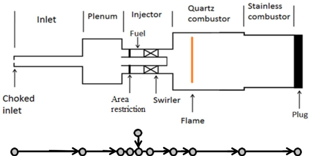
**Figure 4: a) Simplified geometry of the PSU test rig used in the acoustic network model; b) Connections of ducts – straight lines indicate ducts, arrows indicate flow direction, and circles indicate nodes where ducts are connected and boundary conditions are defined**
