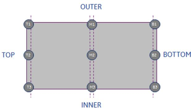
**Figure 2 Cut up plan for slab**
