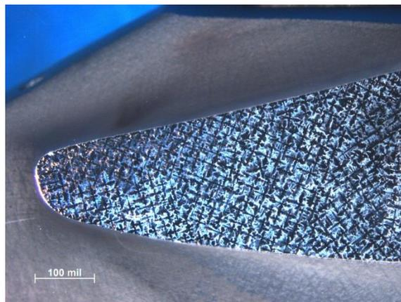
Figure 5 Blade tip cross section
