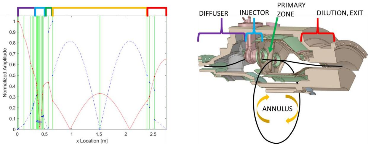
**Figure 5:** Valid Self-Excited Mode Shape (Red: Pressure, Blue: Volume Velocity)
