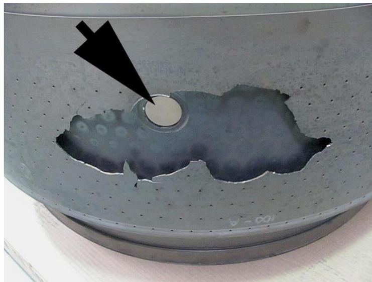
**Figure 1:** *Combustion Liner Damage Caused by Combustion-Induced Oscillations*
