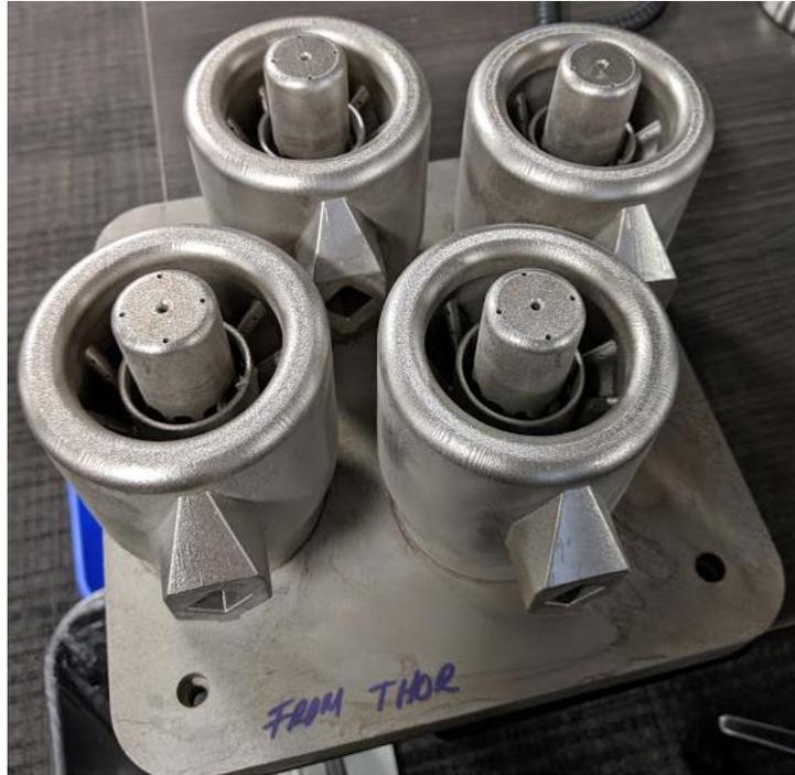
**Figure 3:** Preliminary Injector Head Results from Additive Manufacturing Process
