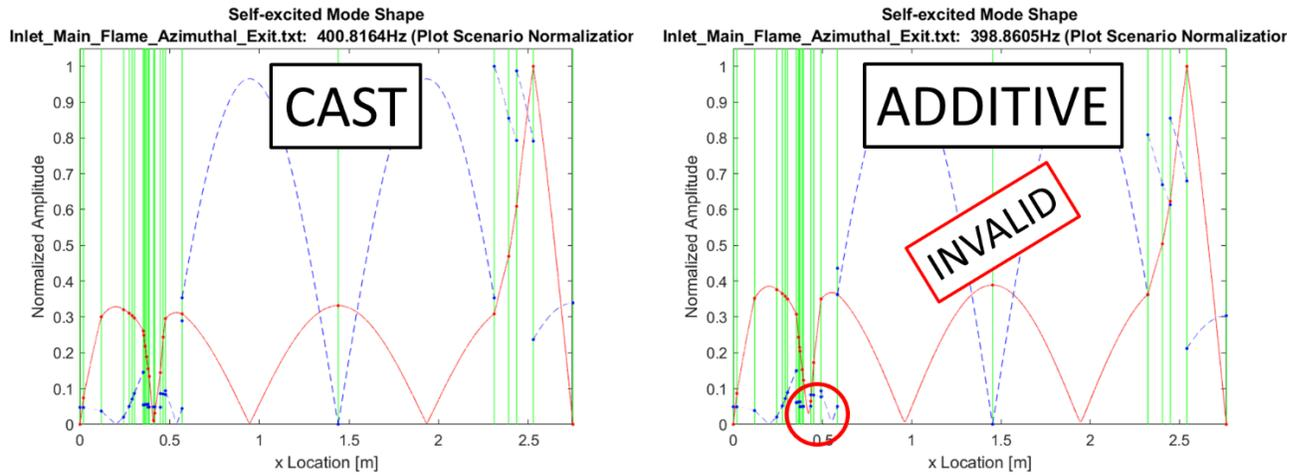
**Figure 8:** 400 Hz Mode Shapes on Cast and Additive Models
