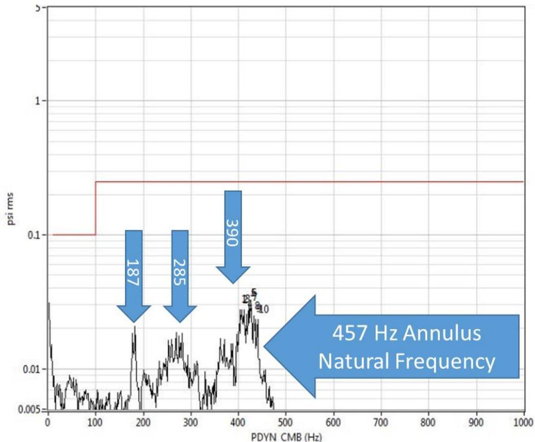
**Figure 7:** Spectral Test Results for Model Validation
