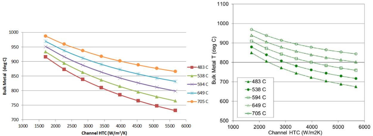
Figure 7: Calculated (left) and Bunker (right) substrate mean temperature as a function of coolant temperature and channel HTC with a constant cavity HTC of 284 W/m<sup>2</sup>/K
