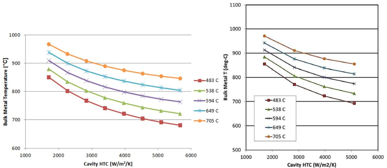
Figure 3: Calculated (left) and Bunker (right) substrate mean temperature as a function of cavity HTC and coolant temperature
