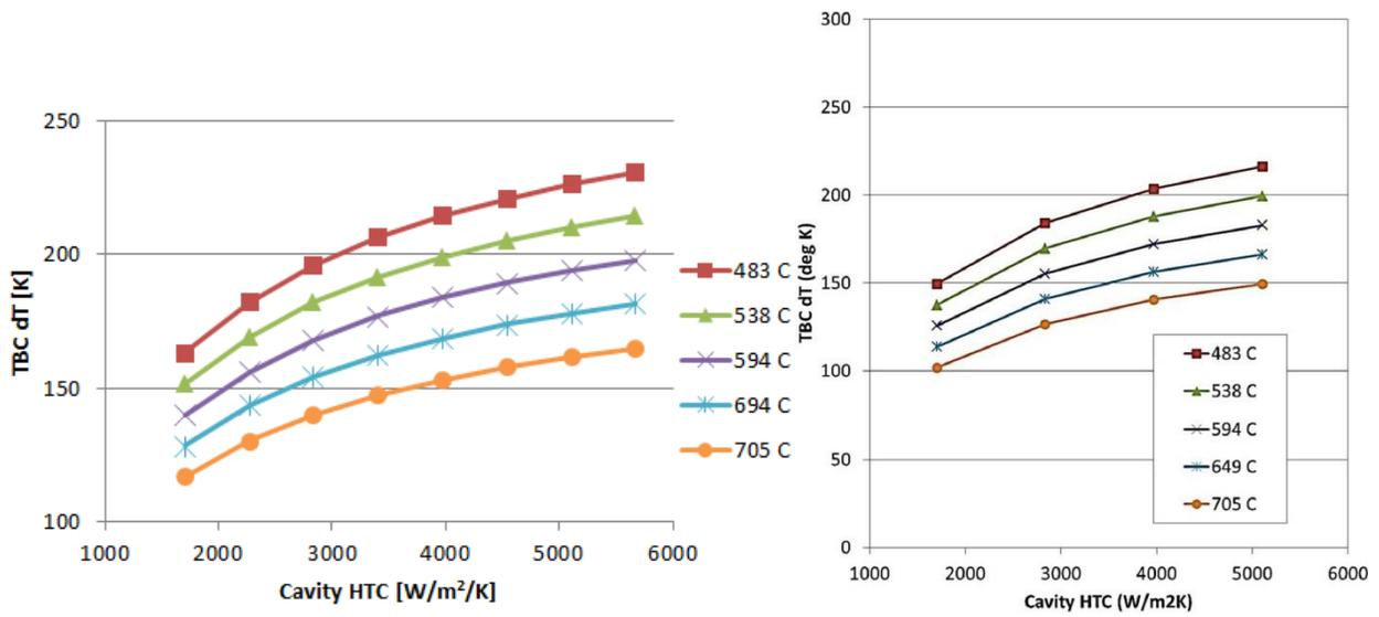
Figure 4: Calculated (left) and Bunker (right) TBC temperature gradient as a function of cavity HTC and coolant temperature
