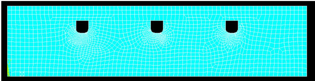
Figure 6: Meshed geometry for the micro cooling heat transfer analysis inside of ANSYS Mechanical APDL
