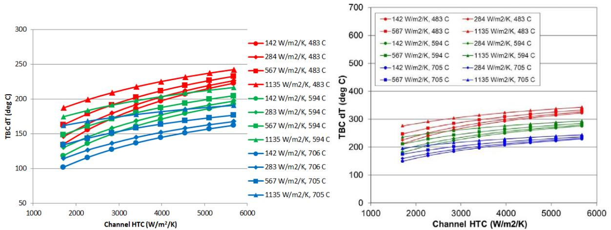
Figure 9: Calculated (left) and Bunker (right) TBC temperature gradient as a function of channel HTC, cavity HTC, and coolant temperature
