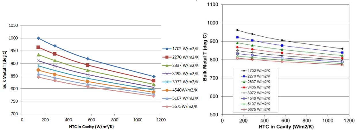
Figure 8: Calculated (left) and Bunker (right) substrate mean temperature as a function of channel HTC and cavity HTC with a constant coolant temperature of 922 K
