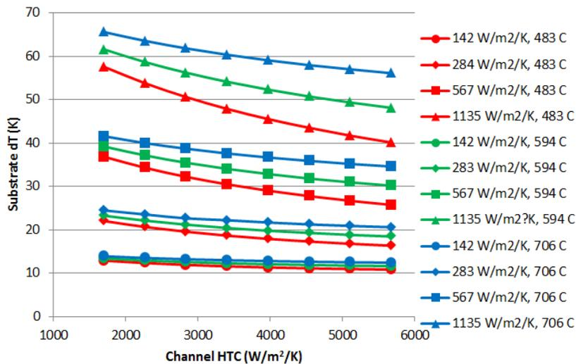
Figure 10: Calculated substrate temperature gradient as a function of channel HTC, cavity HTC, and coolant temperature
