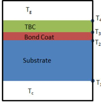
Figure 2: Simplified wall section of an airfoil representing a bulk cooling scheme
