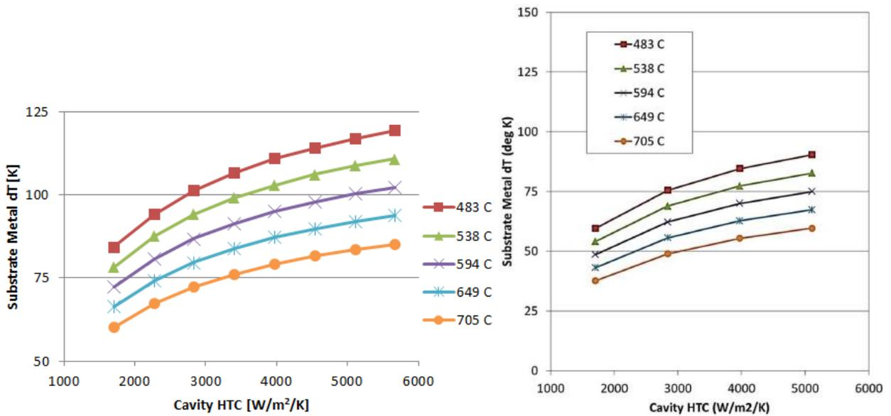
Figure 5: Calculated (left) and Bunker (right) substrate temperature gradient as a function of cavity HTC and coolant temperature
