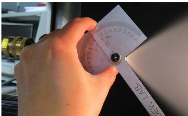
Figure 1: Measuring Spray Angle by Hand
