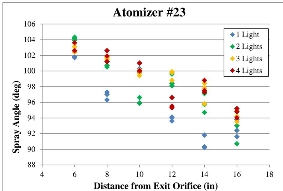
Figure 11: Light Intensity Experiment
