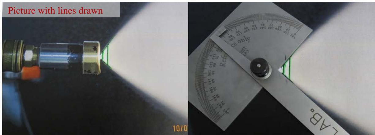
Figure 2: Measuring Spray Angle by Pictures
