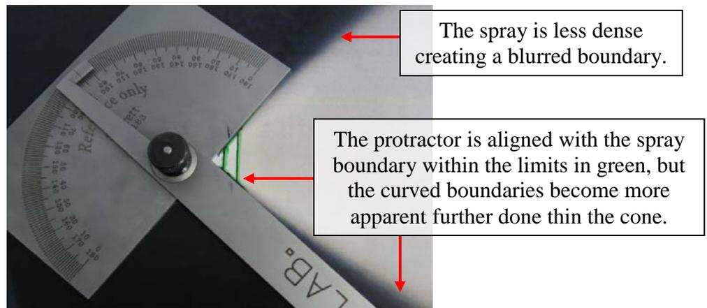
Figure 6: Spray Cone Characteristics
