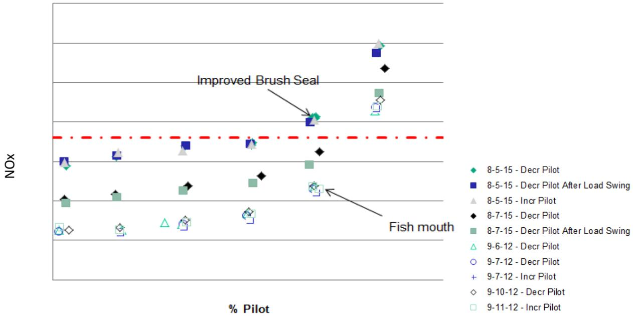
**Figure 3:** Full Load NOx vs Pilot (NOx values redacted)
