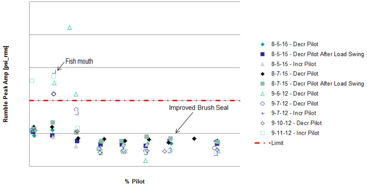
**Figure 5:** Full Load Rumble vs Pilot
