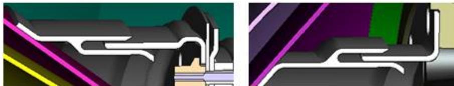
**Figure 1:** Outer fish mouth seal (left), Inner fish mouth seal (right)
