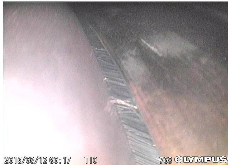
**Figure 9:** Borescope of brush seal
