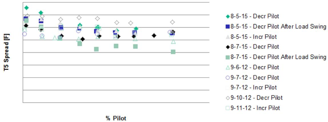
**Figure 7:** Full Load T5 spread vs Pilot (solid symbols represent the brush seal)
