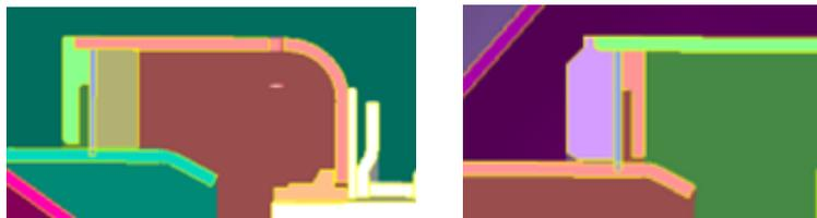
**Figure 2:** Outer brush seal (left), Inner brush seal (right)
