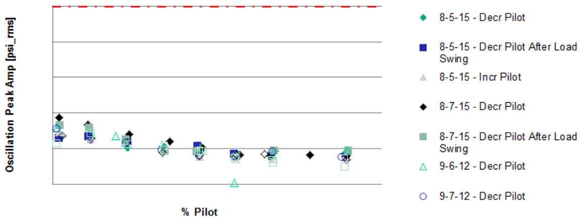
**Figure 8:** Full load Oscillation vs Pilot (solid symbols represent the brush seal)
