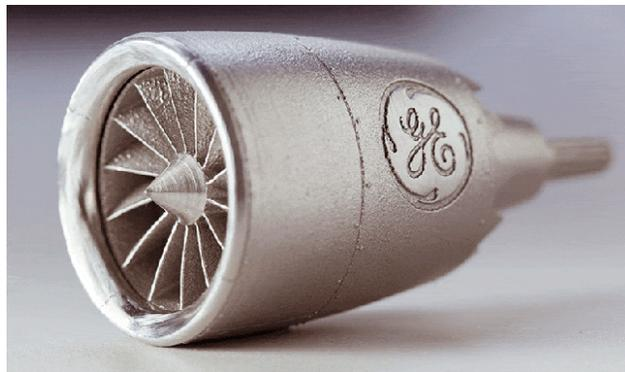
*Figure 1: Capabilities of DMLM. Model of a GENx jet engine*
