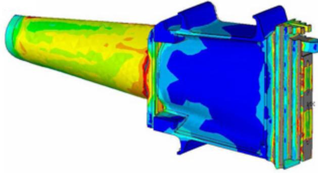
*Figure 3: Example of Von Mises Stress of a blade*
