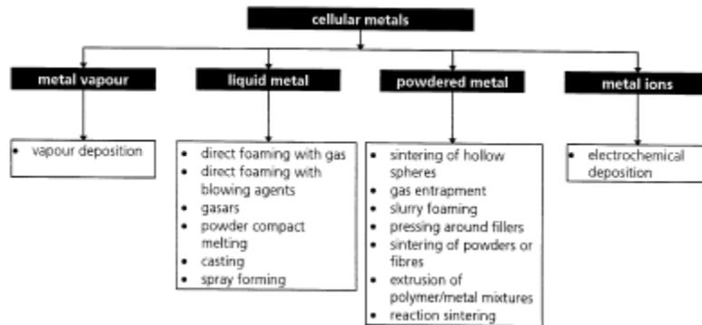
Figure 1. Methods for forming metallic foams [2].
