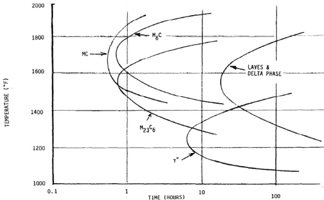
Figure 3. TTT diagram for A625 at high temperatures [11].
