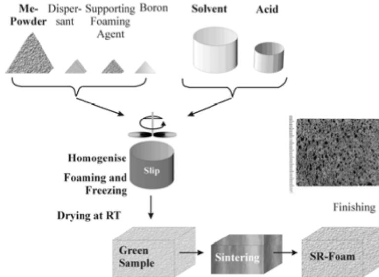
Figure 2. Slip Reaction Foam Sintering (SRFS) process [5].
