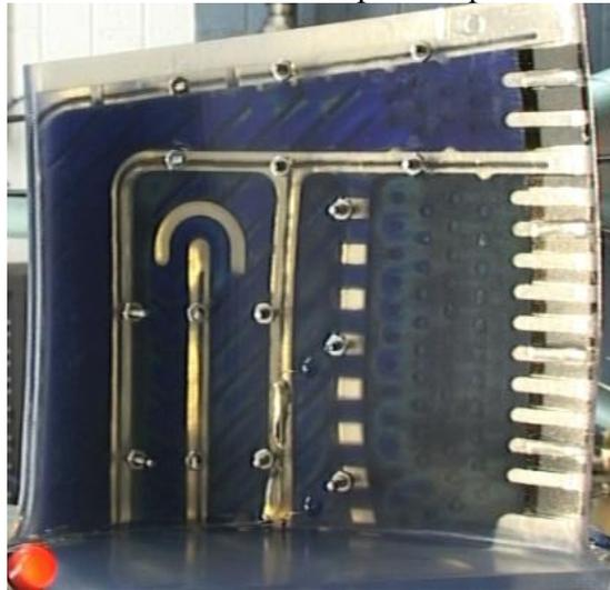
**Figure 7: Transient Liquid Crystal Test of Multi-Pass Serpentine Blade**
