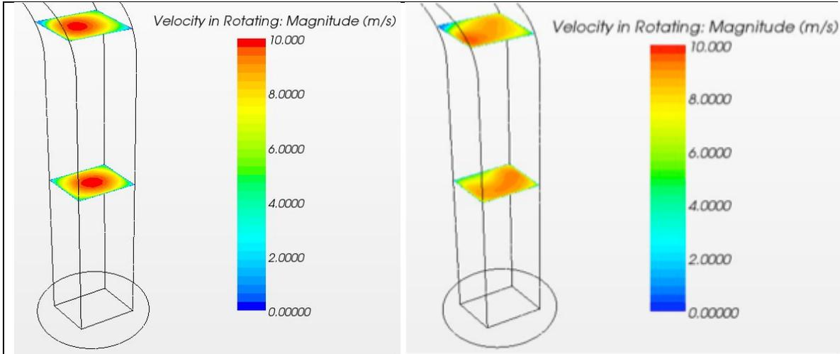
**Figure 5: Velocity Contours in Inlet Section of Test Section for Static Conditions (Left) and Rotating Conditions (Right)**
