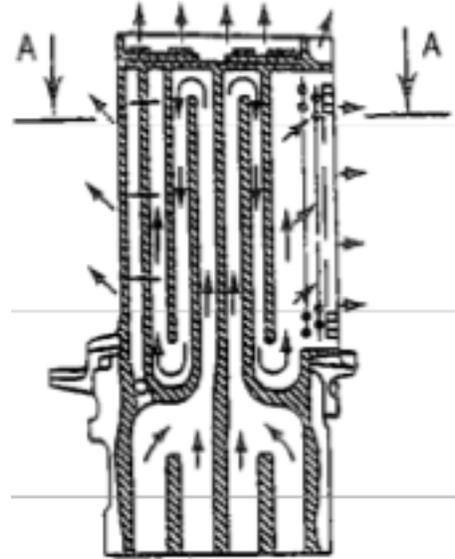
**Figure 1: First Stage Blade - Multi-Pass Serpentine Channel**
