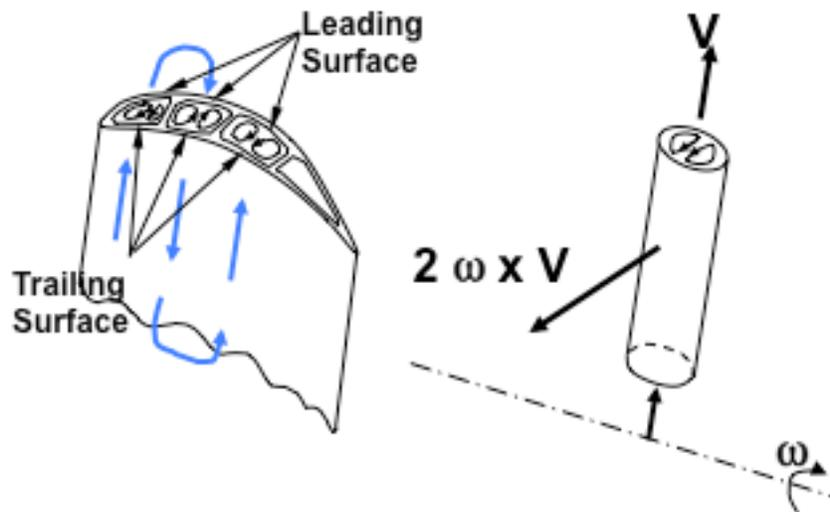
**Figure 2: Secondary Flow Vortices due to Rotation Effects**
