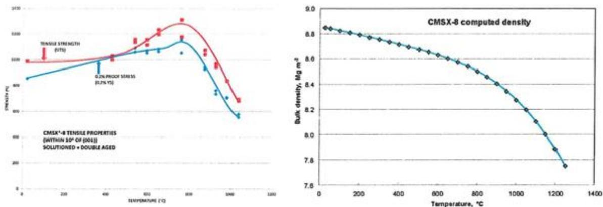
Figure 1 Selected properties of CMSX-8 (B/C) analyzed and used to create estimated design curves for initial alloy selection.<sup>1</sup>
