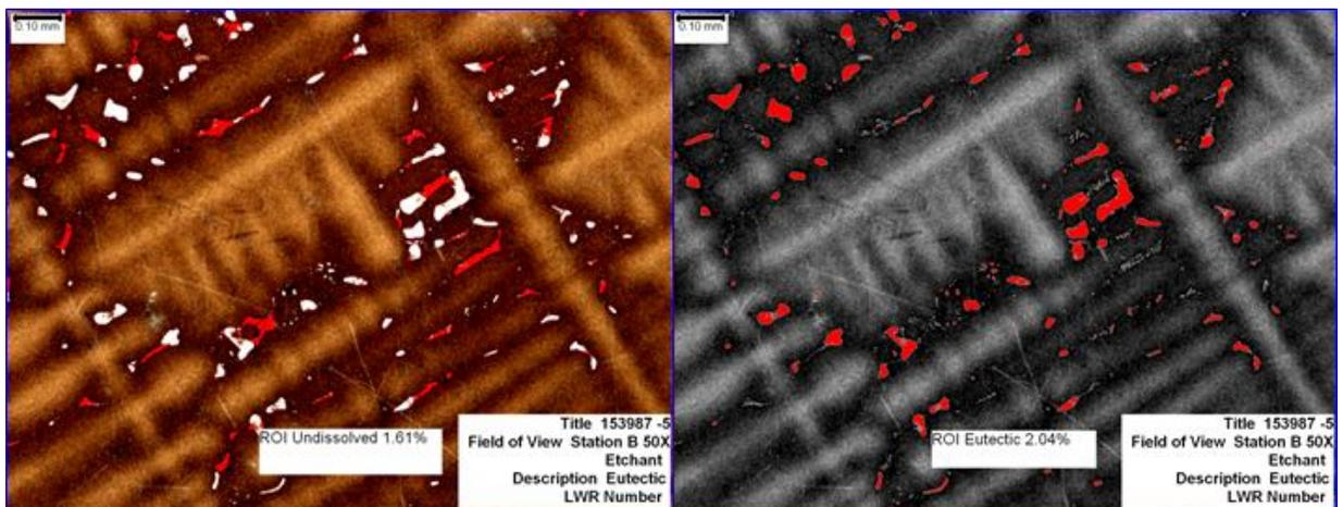
Figure 4 Using the PAXIT Software to analyze gamma prime eutectic phase percentages and large partially solutioned gamma prime in PWA1484.
