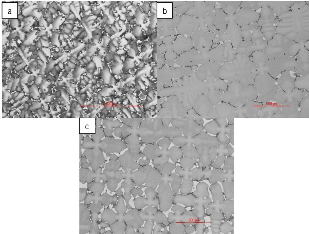
**Figure 2** The as-cast microstructures of the three alloys chosen for study: a) CMSX-486, b) PWA1484 and c) CMSX-8 (B/C).
