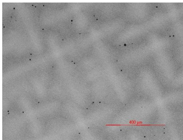
**Figure 3** PWA1484 heat treated at 1330C for 4 hours.
