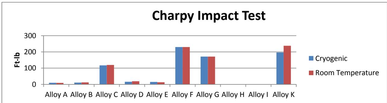
**Figure 10:** Charpy Impact Test of Examined Alloys
