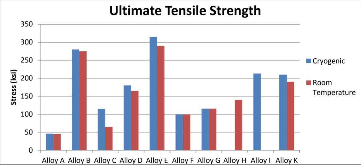
**Figure 6:** Tensile Strength of Examined Alloys
