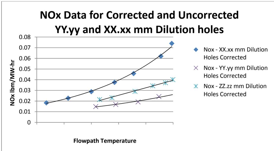
Figure 5: NOx emissions for each combustor
