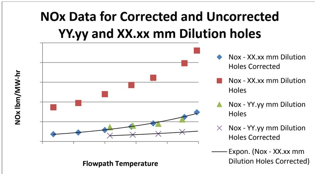
**Figure 3:** NOx emissions from XX.xx mm and YY.yy mm dilution holes, with and without COGEN credit
