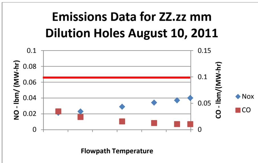
**Figure 4:** Emissions for ZZ.zz mm dilution holes (with COGEN)
