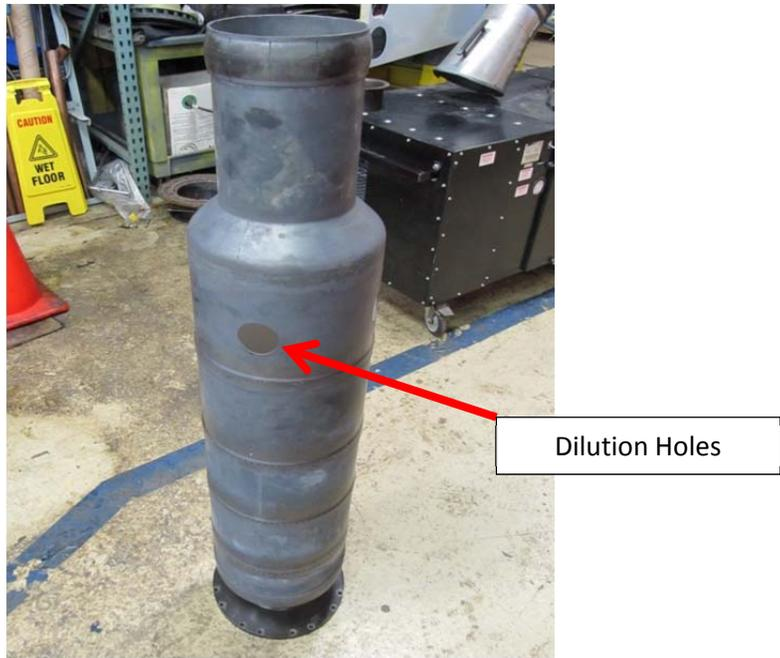
**Figure 1:** Combustor for first emissions tests (Dilution Hole Size  $\varnothing$  XX.xx mm)
