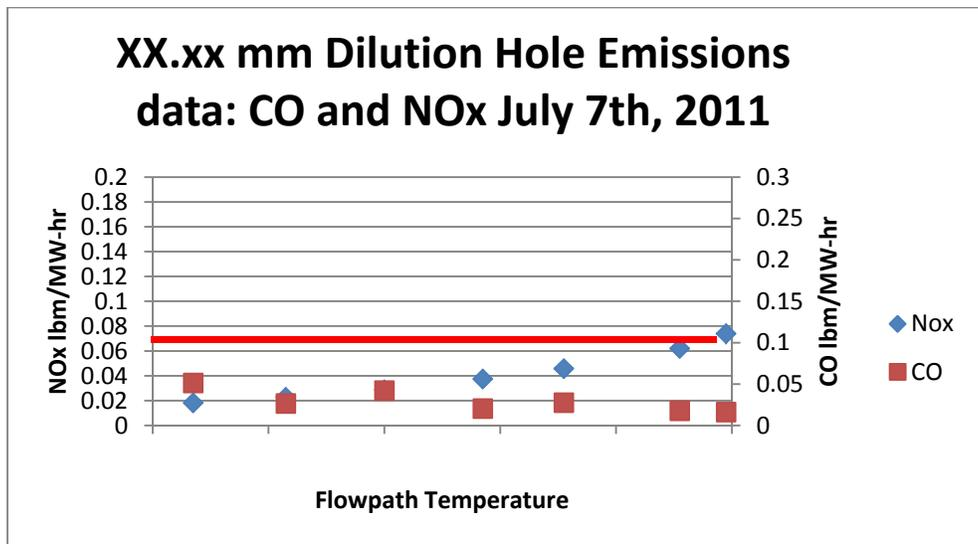
**Figure 1:** Emissions data for XX.xx mm Dilution Hole Size
