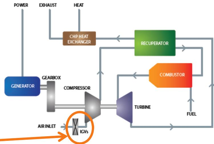
New key feature: Inlet guide vanes improve part-load conditions
